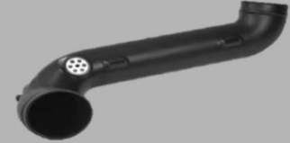
PRODUCT NAME: VOLVO INTERMEDIATE PIPE CATEGORY: DUCTS & FILTERS
