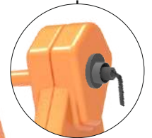
Tighten the bolt with allen key
